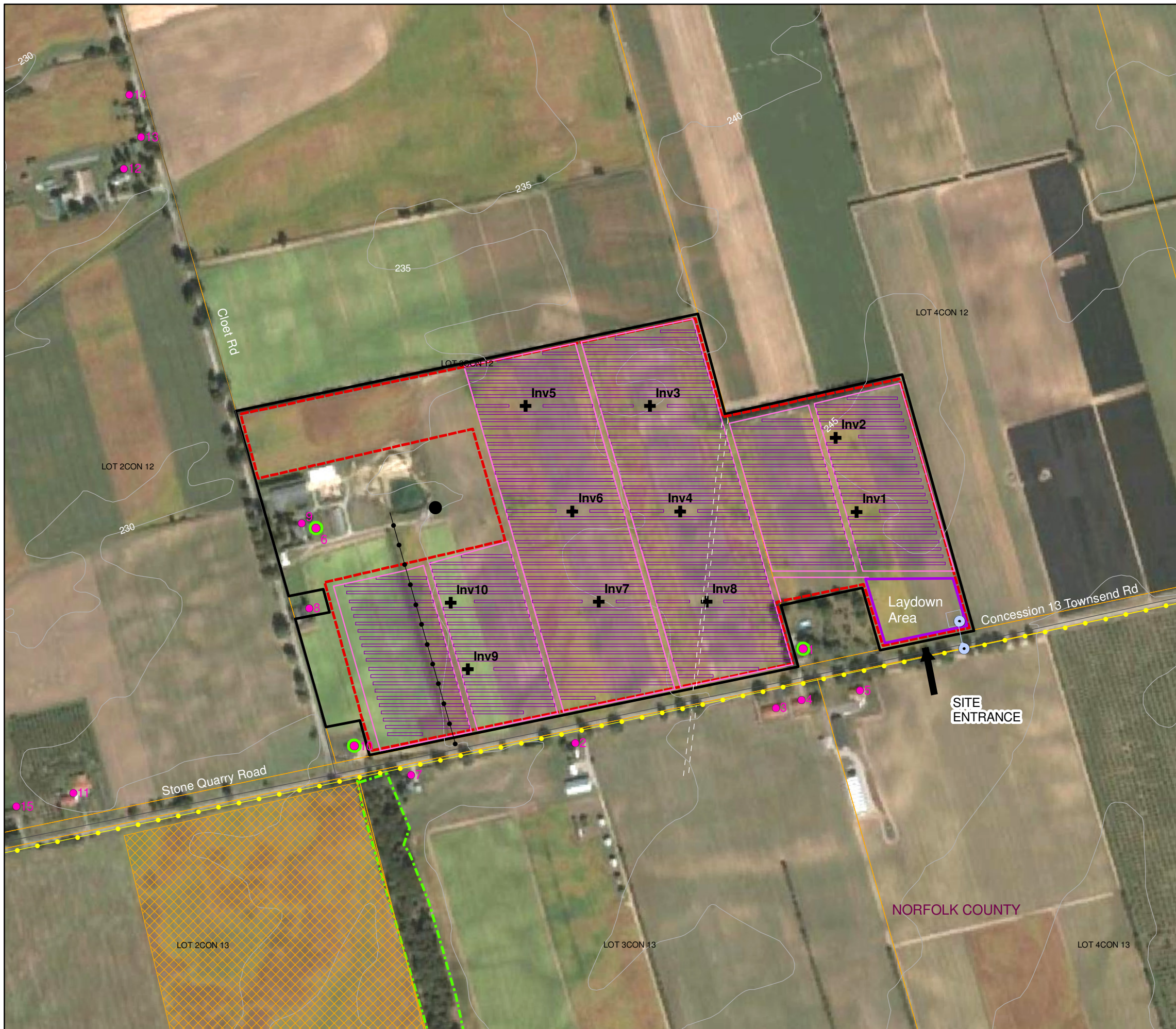
Figure 2.1 Axio Power Canada Inc./SunEdison Canada Norfolk Bloomsburg TS - Solar Energy Project Site Layout Plan
